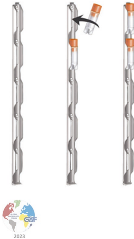
Fig. 8.5 Proper placement of cryovials into cryocanes
