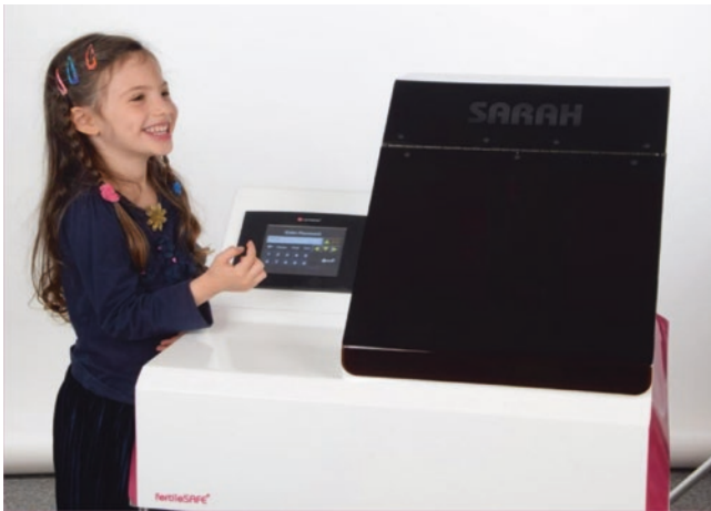
Fig. 49.2 The automatic vitrification device Sarah by FertileSAFE
