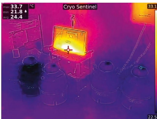
Fig. 46.2 A failing dewar showing clear signs of vacuum failure even at room temperature
